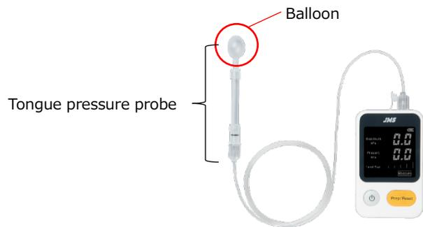
JMS Tongue Pressure Measurement Device
